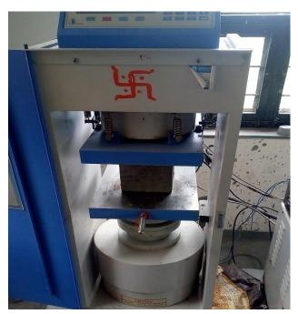
Fig. 6 Compressive strength testing machine
