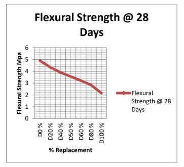
Fig. 12 Graph b/w % Replacement and Flexural strength @ 28days
