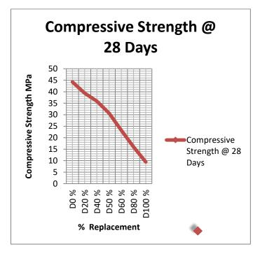
Fig. 9 Graph b/w % Replacement and compressive strength @ 28days
