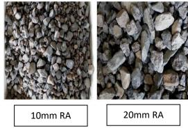
Fig. 4 Recycled Aggregate extracted in nominal size
