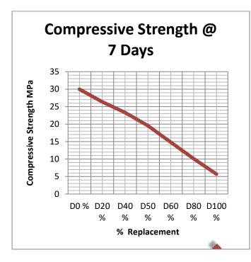
Fig. 8 Graph b/w % Replacement and compressive strength @ 7days
