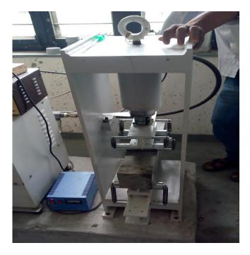
Fig. 7 Flexural strength testing machine
