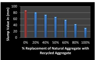
Fig. 5 Graph for Slump value at different % replacement of RA with NA
